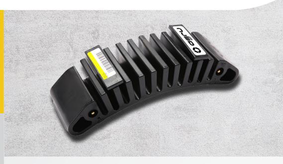
AGRU Flex Restraint is a flexible bar for electrofusion welding onto PE 4710/PE 100/PE 100-RC pressure pipes to absorb high forces to prevent axial movement. This specialized fitting is placed onto the pipe with a tensioning belt and homogenously electrofusion welded in accordance with AGRU installation guidelines based on DVS 2207-1.
