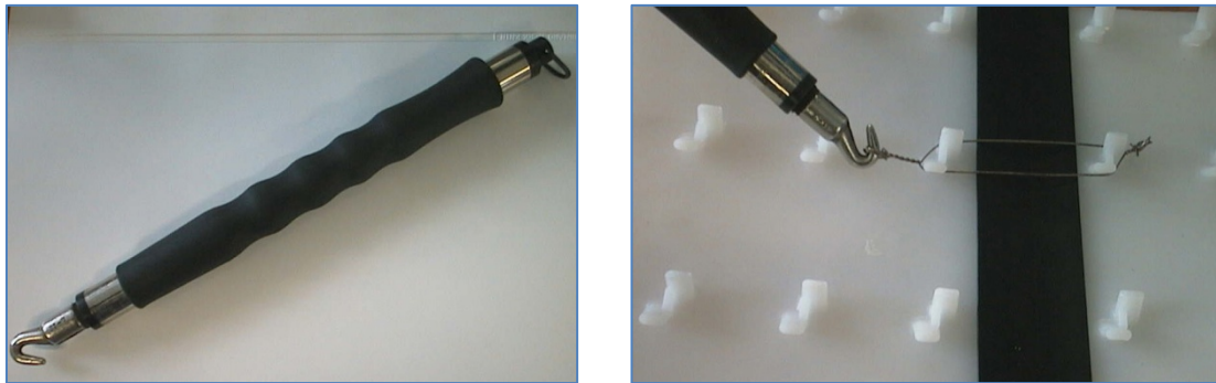
(Example: Connection of CPL by means of wire loops at every 6 th row of studs)
