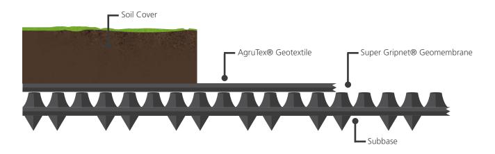
HDPE and LLDPE Super Gripnet® applications include projects where containment, drainage, interface friction and economic dynamics are critical. These projects include landfill closures, containment facilities, oil & gas applications, minining reclamation projects, to name a few.
