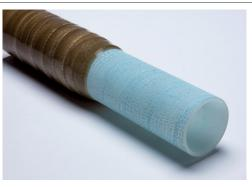
The PVDF HV-Liner from AGRU is an economical alternative to traditional fabric backed pipes. The surface-treated PVDF pipe has a three-dimensional surface structure which provides an optimal bonding to the FRP pipe. The piping systems are available in PVDF, PVDF-FLEX, and PVDF-el ESD. The pipes can be produced in diameters from 20–400 mm.
