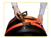
After the cooling time is over pull the function slider of the ratchet lever and move it 180° into the end position in order to open the tension belt.
