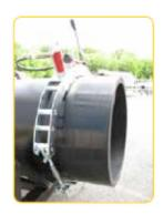
In order to ease the coupler's installation, chamfering of the pipe's outside edge on the face to be inserted (0.2" × 45°) is helpful. The pipe's inside edge must not be chamfered. Chips from scraping or cutting must be removed from the pipe.
