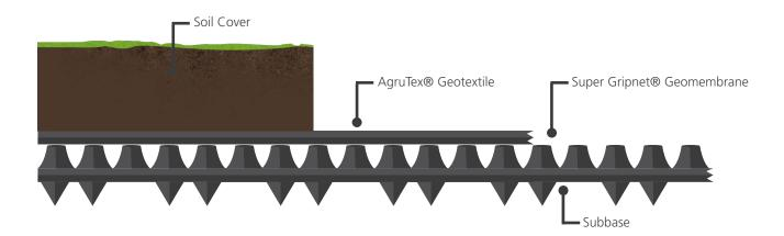
HDPE and LLDPE Super Gripnet® applications include projects where containment, drainage, interface friction and economic dynamics are critical. These projects include landfill closures, containment facilities, oil & gas applications, minining reclamation projects, to name a few.
