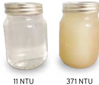
Runoff from a typical 1" rainfall (same site); ClosureTurf (left); traditional soil cover (right)
